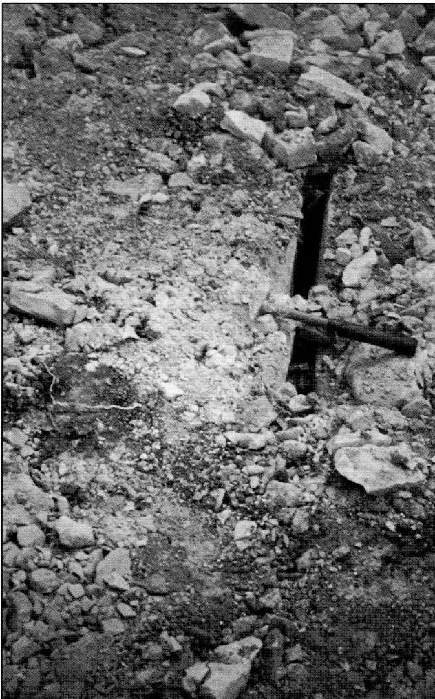
Fig. 7. Joints up to 100mm wide in Lincolnshire Limestone. These trend parallel to the valley side at the top of upper escarpment, and have opened up as a result of cambering of the Limestone.
